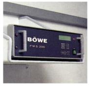
The Perc Measuring System Controls the Residual Solvent Concentration
